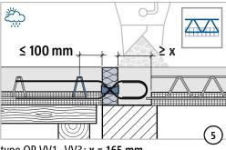
type QP VV1-VV3: **x = 165 mm** type QP VV4-VV6: **x = 230 mm**
