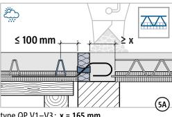
type QP V1-V3: **x = 165 mm** type QP V4-V6: **x = 230 mm** type QP V7-V9: **x = 100 mm**
