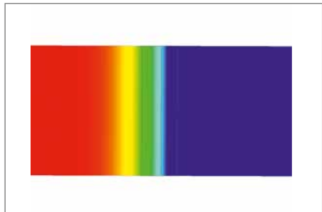
Figure 8b: Top view; this shows a cross-section through the balcony slab presented in 8a. You can clearly see that the heat loss is linear, meaning it remains the same across the entire connection length of the balcony.
