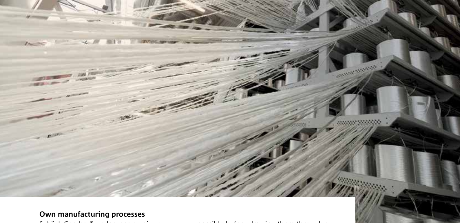
Roving spools and fibre guide for pultrusion ©Fiberline Composites A/S
