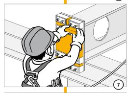
Tit any additional thermal insulation pieces at the head plate of the steel beam between the insulation bodies of Schöck Isokorb® Type S22.
